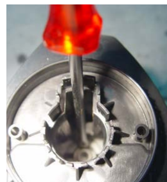
O-Ring at wrong position
