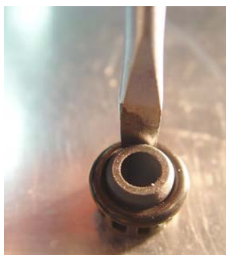
O-Ring at correct position
