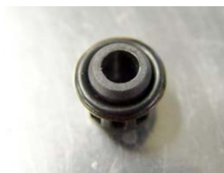
O-Ring at correct position
