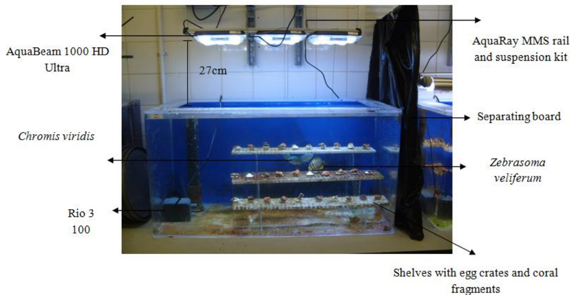
Figure 6.3 LED tank set up
